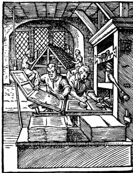
Left in the foreground, a printer removes a printed page from the press. The printer at right is inking the plate. In the background, compositors are using cast type.
